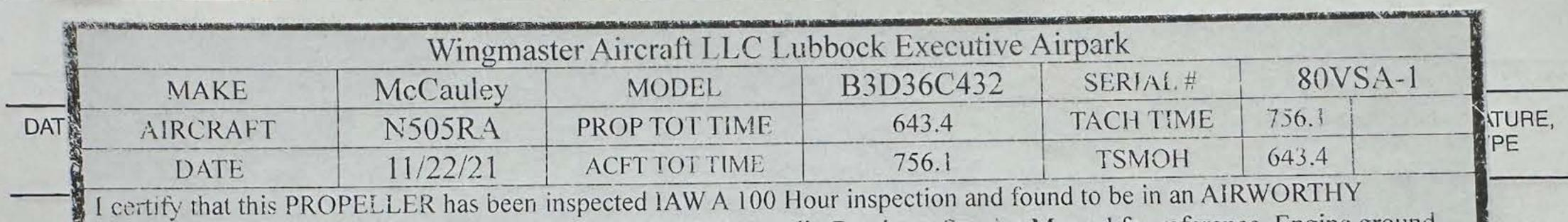
condition. Inspected IAW the scope and detail of Part 43 Appendix D using a Service Manual for reference. Engine ground ran and test flown, no defects noted. See AD summary for compliances.
