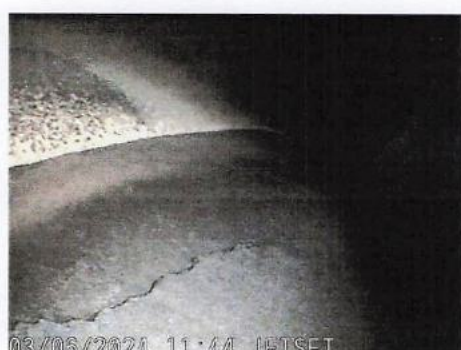
HT Vane Outer Wall Crack
