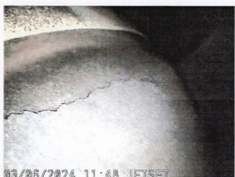
HT Vane Outer Wall Crack
