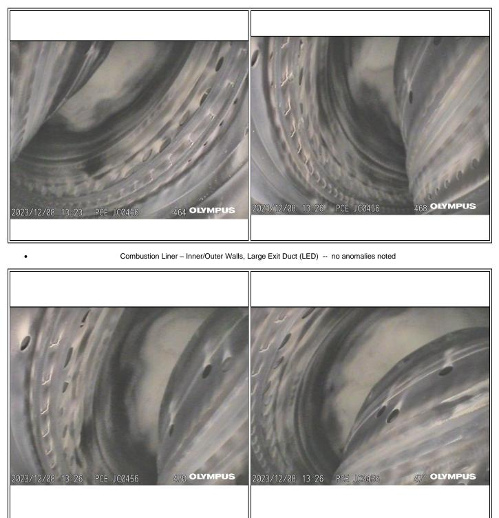
Page 9 <u>NOTE:</u> Given the nature of borescope instrumentation it is often not possible to make observations and examine all areas of an individual engine as part of an evaluation. Based on this limitation, Dallas Airmotive, Inc. cannot and does not warrant its findings for borescope evaluations (pre-purchase and otherwise) against the possibility that hidden damage may exist that was not observable and reported by our technician at the time of the evaluation.
