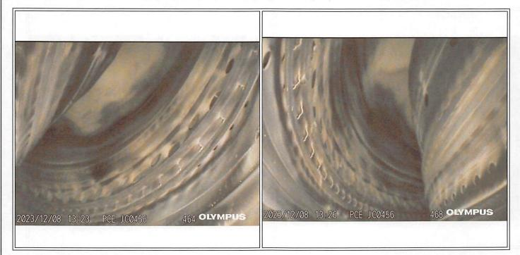
Combustion Liner - Inner/Outer Walls, Large Exit Duct (LED) -- no anomalies noted
