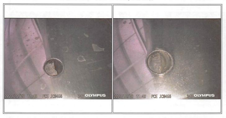
Inlet Case – several rivets noted with missing/broken head(s)
