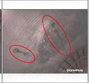
Low Compressor (Fan) - typical, 1 blade exhibiting previous repair
