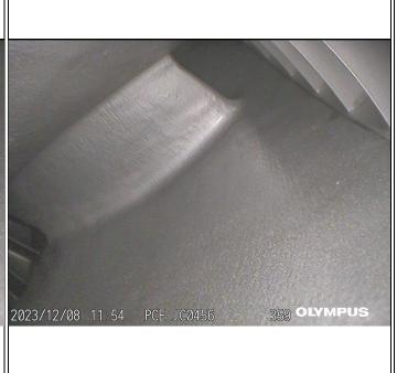
Impeller - main blade & mid-span - no anomalies noted
