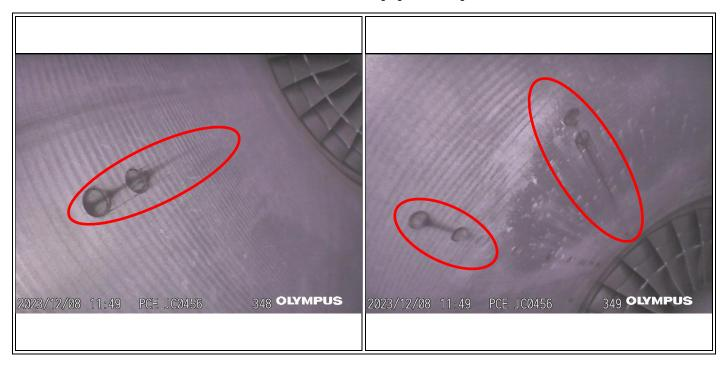
Low Compressor (Fan) – typical, 1 blade exhibiting previous repair
