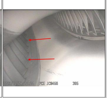
Combustion Liner – Inner/Outer Walls, Large Exit Duct (LED) -- no anomalies noted
