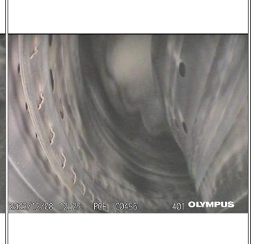
Combustion Liner – Inner/Outer Walls, Large Exit Duct (LED) -- no anomalies noted
