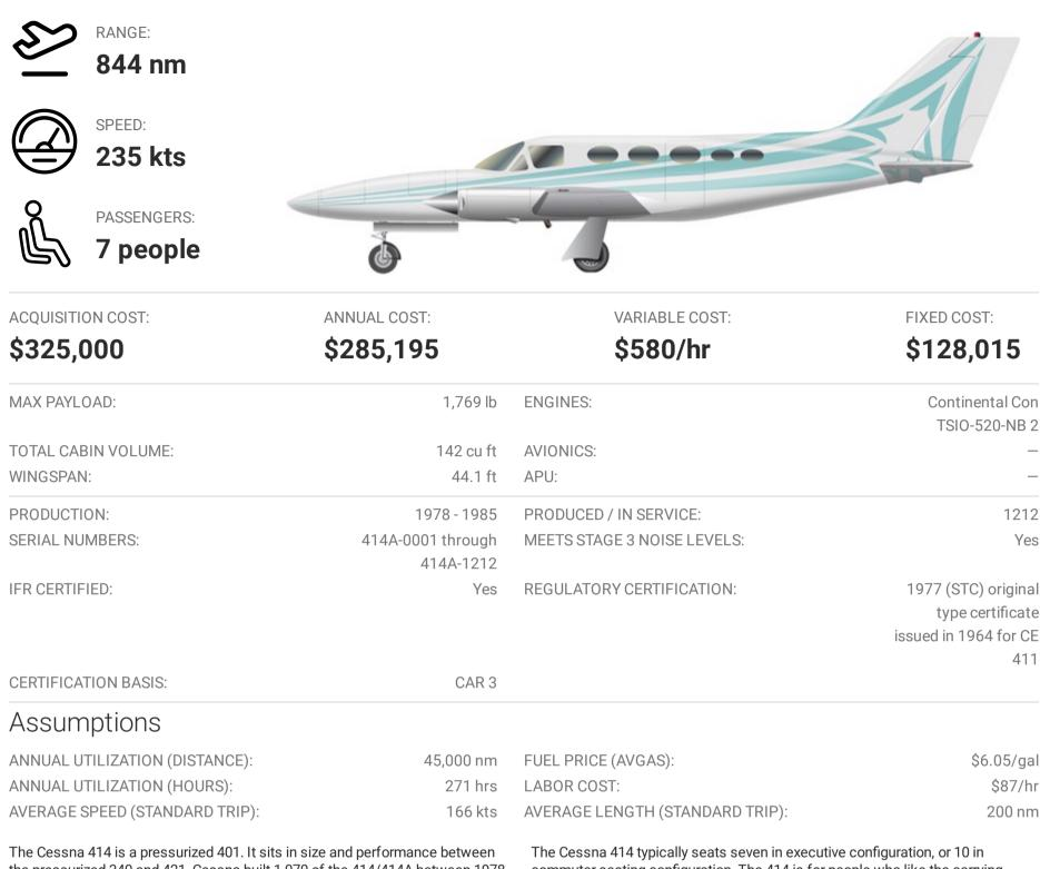
the pressurized 340 and 421. Cessna built 1,070 of the 414/414A between 1978 and 1985. The difference between the 414 and the 414A is the 414s have tip tanks and a short nose while the 414A is longer, has sealed wings, and has the longer nose from the 421. Two 310 hp Continentals power the 414 series.
